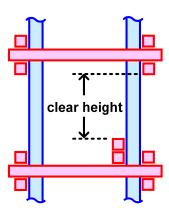
Figure 5. The definition of a clear floor height.
