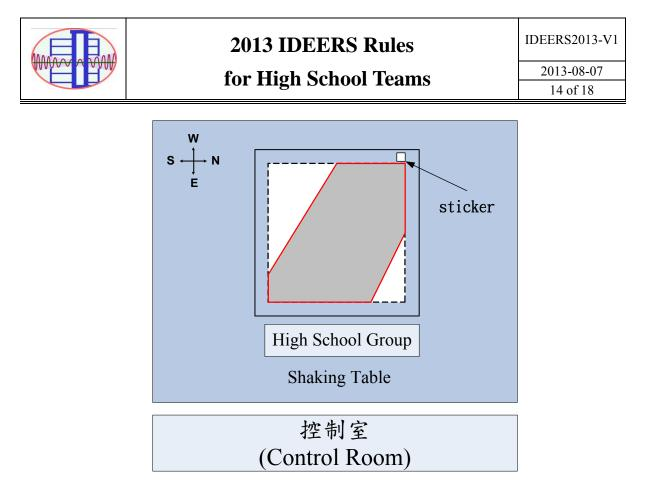
Figure 14. The orientation of the model fixed on the shaking table.
