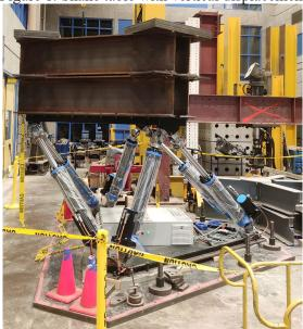
Figure 2. Shake table with horizontal displacement
