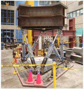
Figure 1. Shake table with vertical displacement
