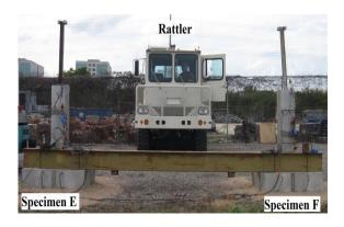
Figure 3. Test Setup of 3D periodic foundation.
