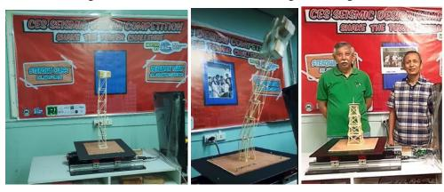
Figure 10. Testing the Stick Towers on the Shake Table
