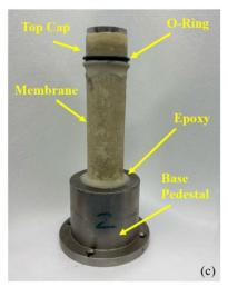
Figure 2. (a) Vesicular basalt; (b) Aphanitic basalt; and (c) Basalt specimen setup with specimen glued to the base pedestal and top cap and covered with a membrane.
