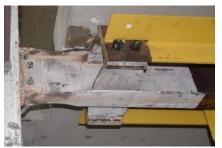
Figure 5 Column base, SBRB connection, and RBS after all tests
