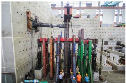
Figure 2. Photo of full-scale cruciform subassembly with lateral support system at NCREE.
