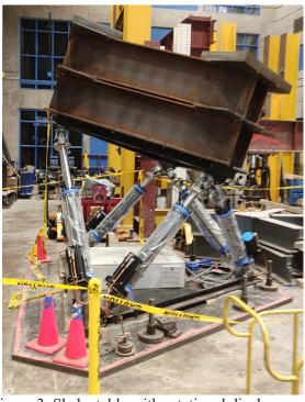
Figure 3. Shake table with rotational displacement
