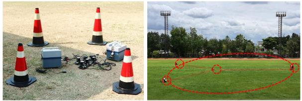
Figure 2. Microtremor equipment and arrangement of array observation
