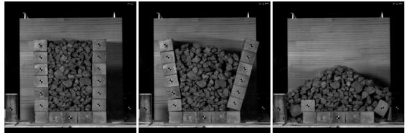
(c) Small crushed stones (8Hz, collapsed at 160gal)
