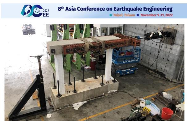
Figure 2 Setup of hybrid simulation test
