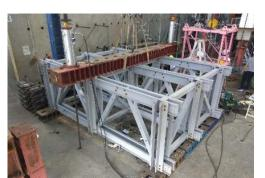
Figure 3. Experimental setup for the flexural test with the applied loading at the mid-span of the specimen.
