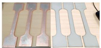
Figure 3. Test pieces of tensile strength testing (conductor/left, enclosure/right)
