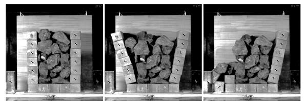
(b) Large crushed stones (2Hz, collapsed at 114gal)
