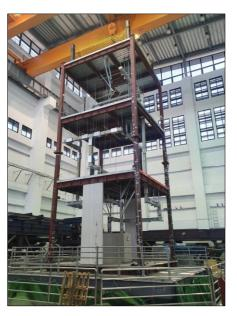
Figure 4. The three-story test frame
