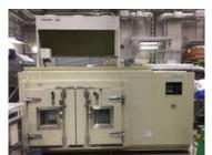
Figure 4. Ozone accelerated deterioration testing machine
