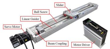
Figure 6. Mechanism of the motor-driven ball screw linear guider
