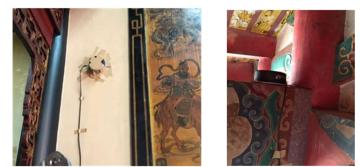
Figure 3. Photograph of vibration sensors installed on wall (left) and adjacent timber frame (right).
