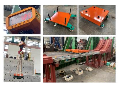
Figure 7. The static load test configuration with flatcars
