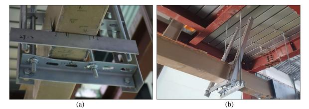
Figure 13. (a) Deformation of the suspended braced frame; (b) Complete failure of the braced frame
