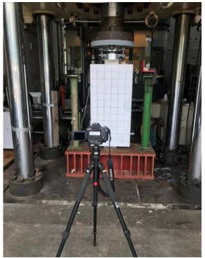
Figure 3. Specimen Arrangement in Compression Testing Machine
