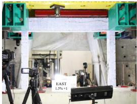
Figure 5. Cracking pattern of specimen PT at the ultimate lateral strength.
