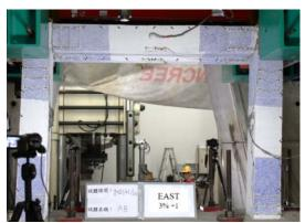
Figure 7. Cracking pattern of specimen AB at the ultimate lateral strength.
