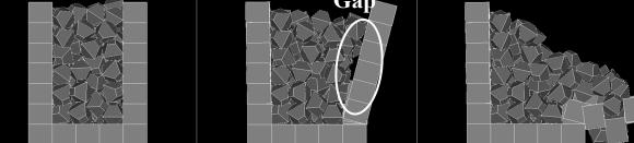
(b)Large crushed stone (8Hz, collapsed at 190 gal)
