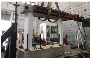
Figure 4. Test setup of the RTHT of the 7-story RC building.
