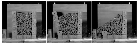
(a) Small crushed stones (2Hz, collapsed at 110gal)
