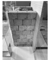
(a) Front view (left-right direction is the excitation direction) Photo 1. Test specimen on the shaking table
