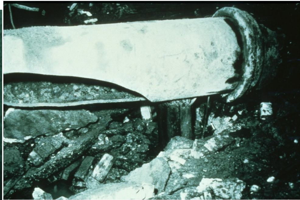
500 mm (20 inch) Cast Iron Main Rupture
