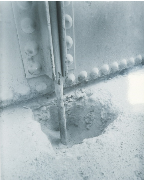
900 mm (36 inch) Concrete Cylinder Pipe Leak
