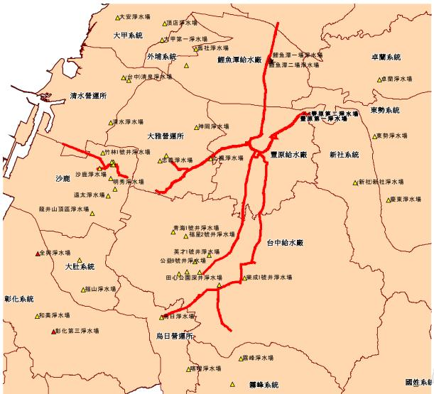
Main transmission pipelines ( $\geq$  800 mm) are used to deliver huge amount of water between two places at a distance
