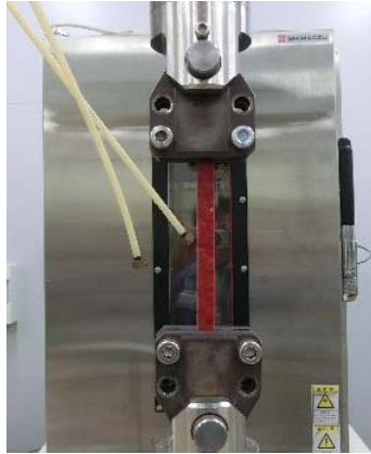
Figure 11. Setup of Level-2 cyclic strain test
