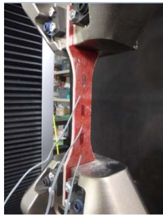
Figure 10. Setup of Level-1 cyclic strain test
