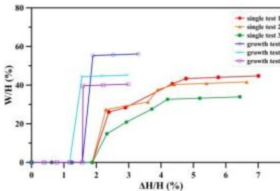
**Fig. 4.** Relationship of offset ratio ( $\Delta H/H$ ) and normalized influenced width ( $W/H$ ) for Type 1 (single) and Type 2 (growth) tests.
