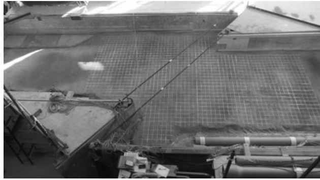
Figure 9. Large-scale split-box test set-ups for the 6-in GX-type ERDIP
