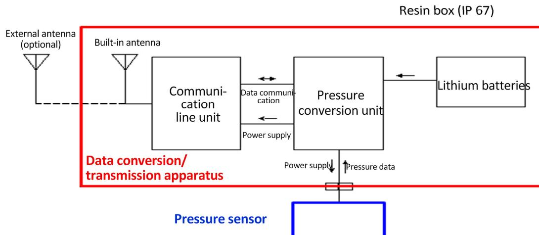
**Figure 3 Configuration of terminal device
