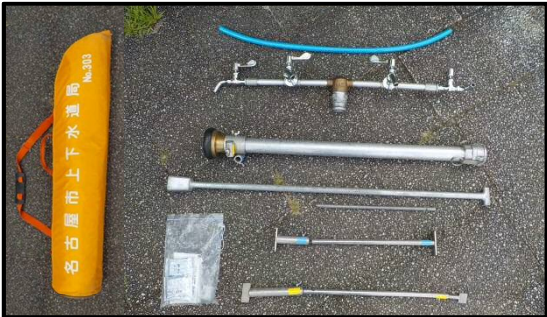
Figure 5. Temporary water faucet
