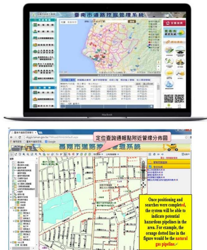
Fig.4 Searching for hazardous pipelines close to the excavation site
