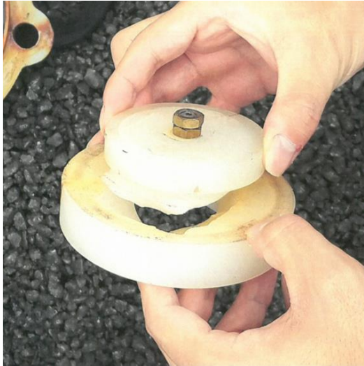
Photo 1. Damaged floating valve body
