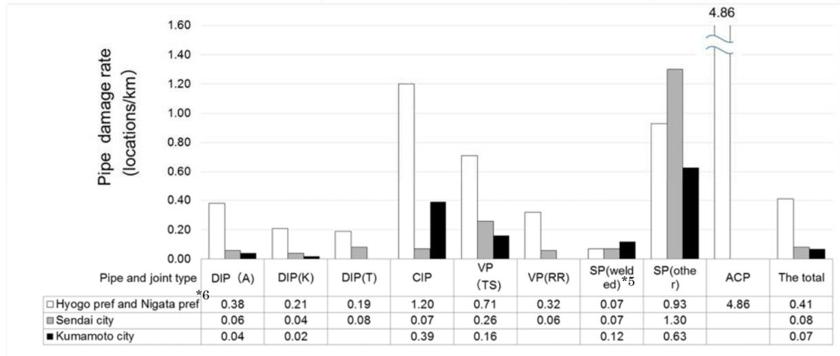
\*5: SP (welded joint) does not include SP with expansion/flange joint.
