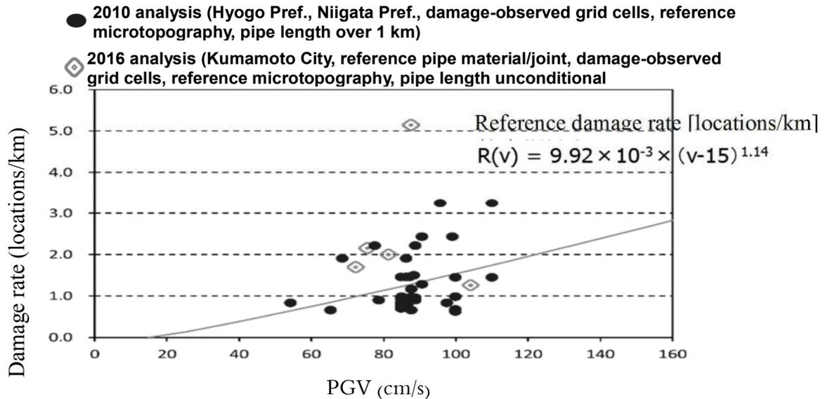
Figure 11. Damage rate of DIP (A) with 100-150 mm diameter in the 2016 Kumamoto Earthquake and in other major earthquakes along with the reference damage rate curve
