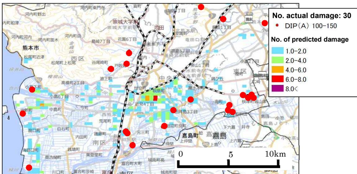
Figure 10. Locations of actual pipe damage and the distribution of estimated pipe damage for the reference pipe material/joint with reference diameter
