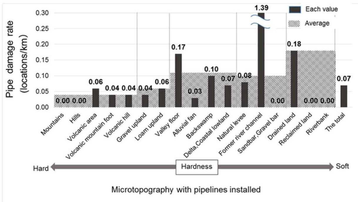
Figure 5. Pipe damage rate by microtopography in Kumamoto City
