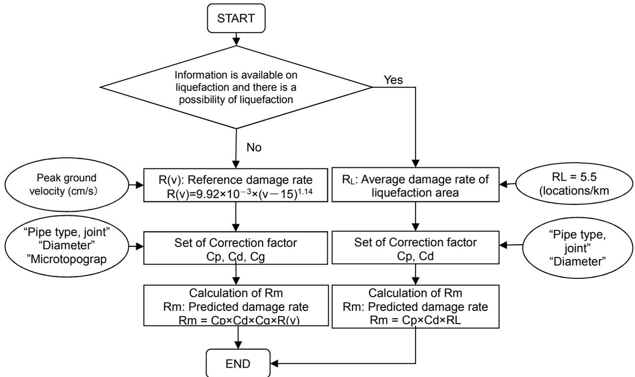
Figure 1. Process of estimating the number of pipe failures in earthquakes
