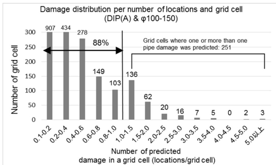
Figure 9. Number of pipe damage estimated by the equation for the reference pipe material/joint with the reference diameter
