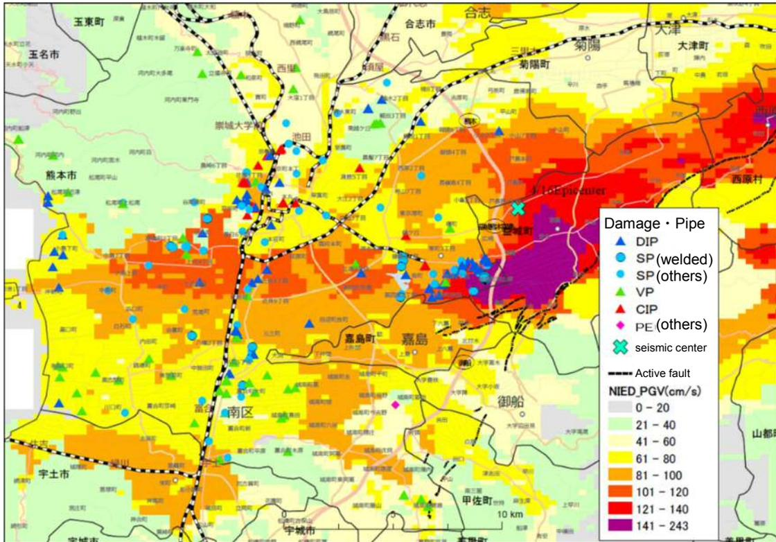
Figure 6. PGV distribution and pipe damage in Kumamoto City from the main shock of the 2016 Kumamoto Earthquake
