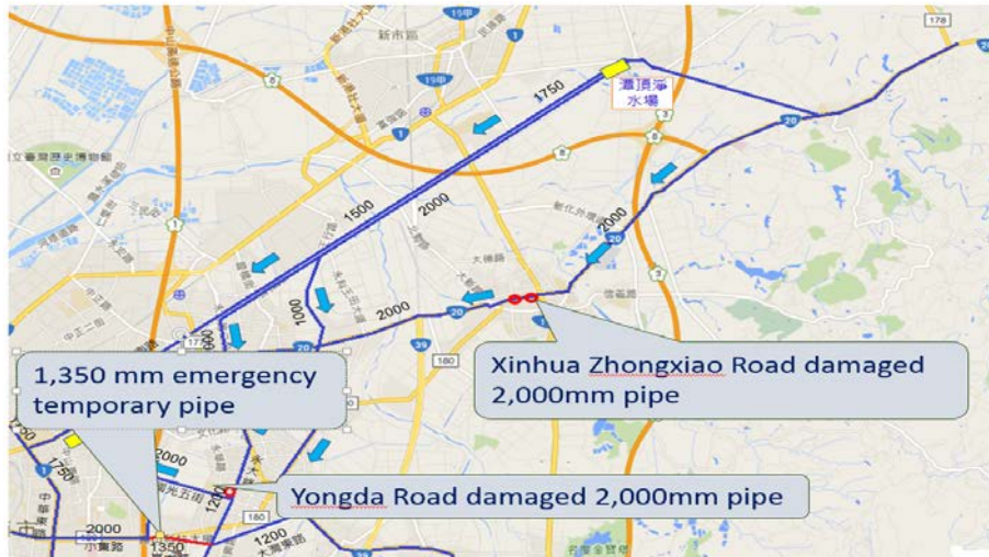
Fig.5 Location of damaged 2,000mm pipe and 1,350 mm temporary pipe
