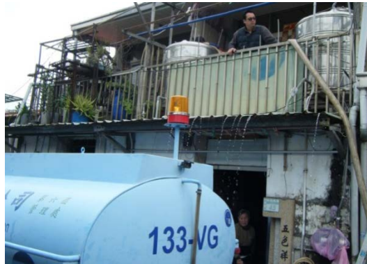
Fig.4 Water tanker injected water into pipeline for supplying water to consumer's water tank
