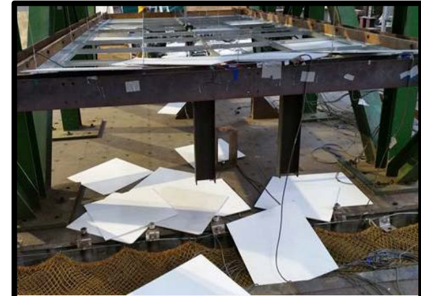
Failure of ceiling panel
