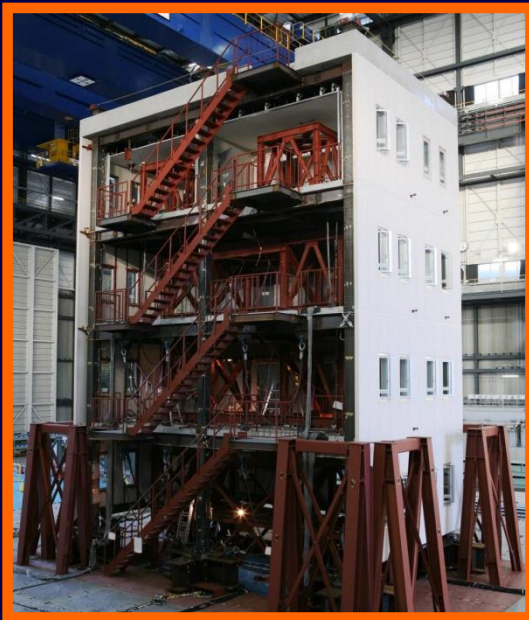
4-Story Bldg. Tested to Collapse
