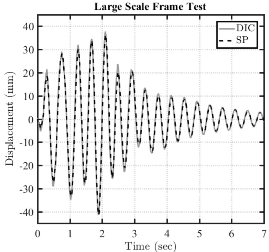
Digital Image Correlation for monitoring large shake table tests at University of Nevada, Reno
