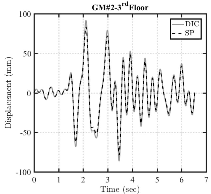
Comparison of results from DIC and conventional measurements (string pots and accelerometers)
