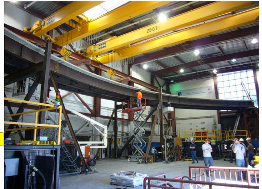
Curved bridge spanning 4 tables, UNR Shake Table Array, Reno, NV, USA
