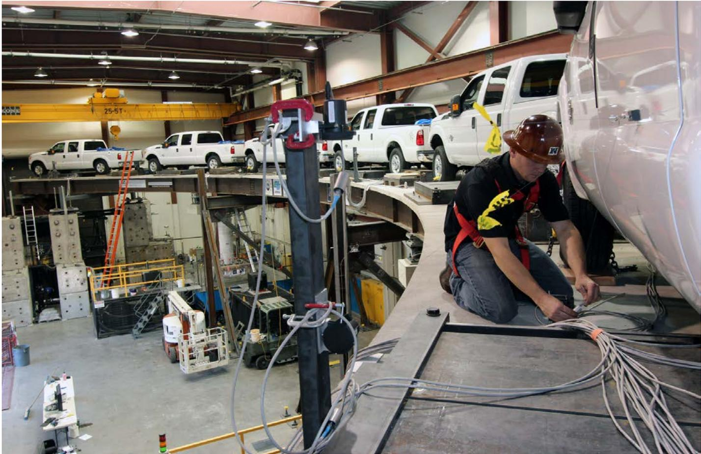
Cabling to accelerometers in trucks on 0.4-scale curved bridge model, University of Nevada Reno, NV, USA
