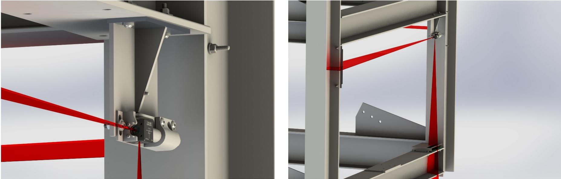
Optical sensors being used to measure interstory drift are monitored wirelessly using laboratory SCRAMNet, University of Nevada Reno, NV, USA
