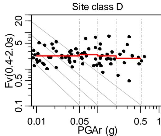
For site class D, the amplitude dependence of the amplifications is slightly observed.
