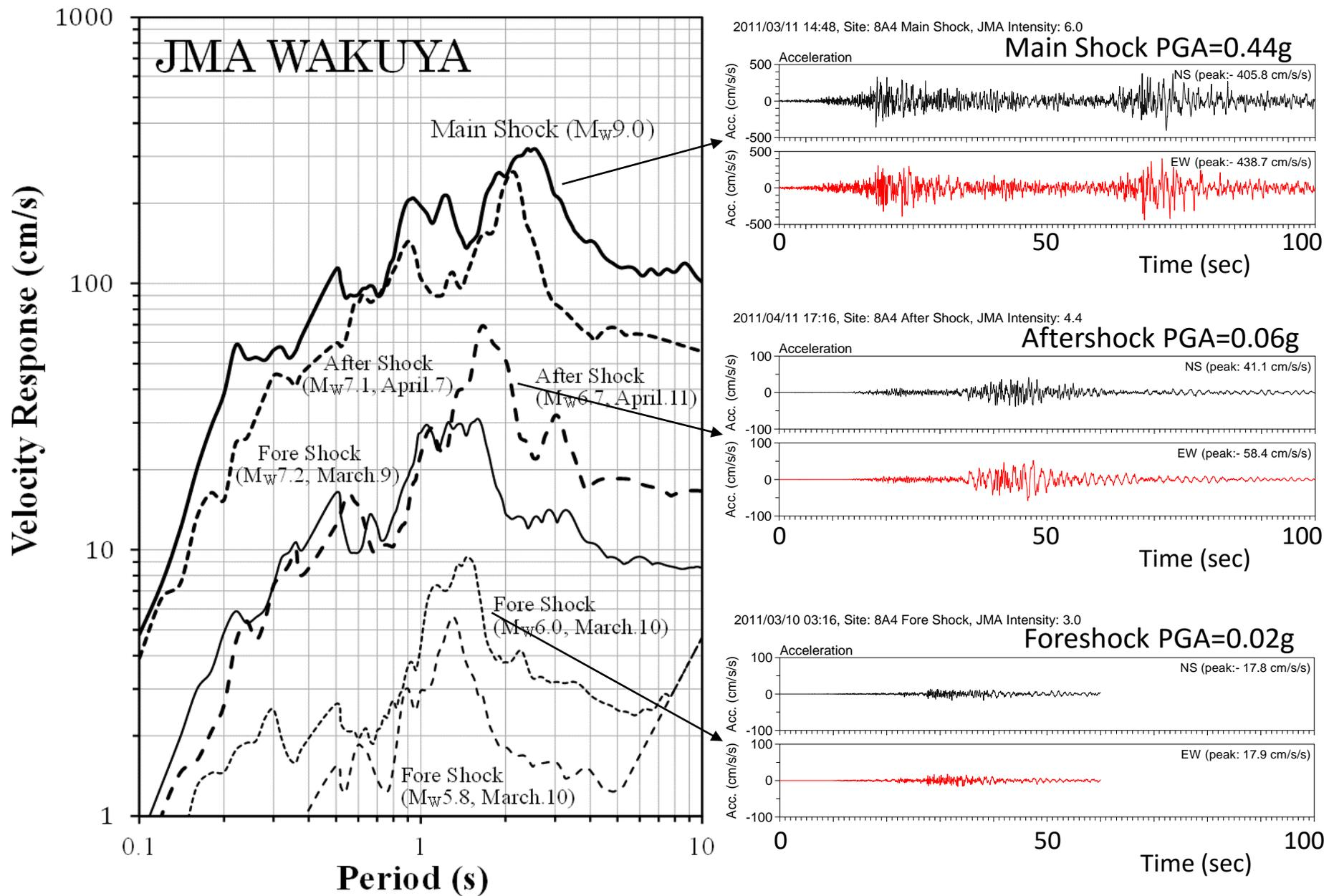
Nonlinear behavior of site response is also found on the records. This figure shows comparison of response spectra of the main shock, foreshock and aftershock records at JMA Wakuya. The site is located on the alluvial lowland, and classified to the site class E.
