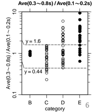
Finally, using the soil profile data and microtremor data, the sites are classified into 30 class B sites, 153 class C sites, 207 class D sites and 77 class E sites.
