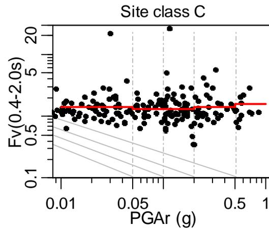
This figure shows the amplifications for short-period Fa and for longer period Fv from the different station pair records.
