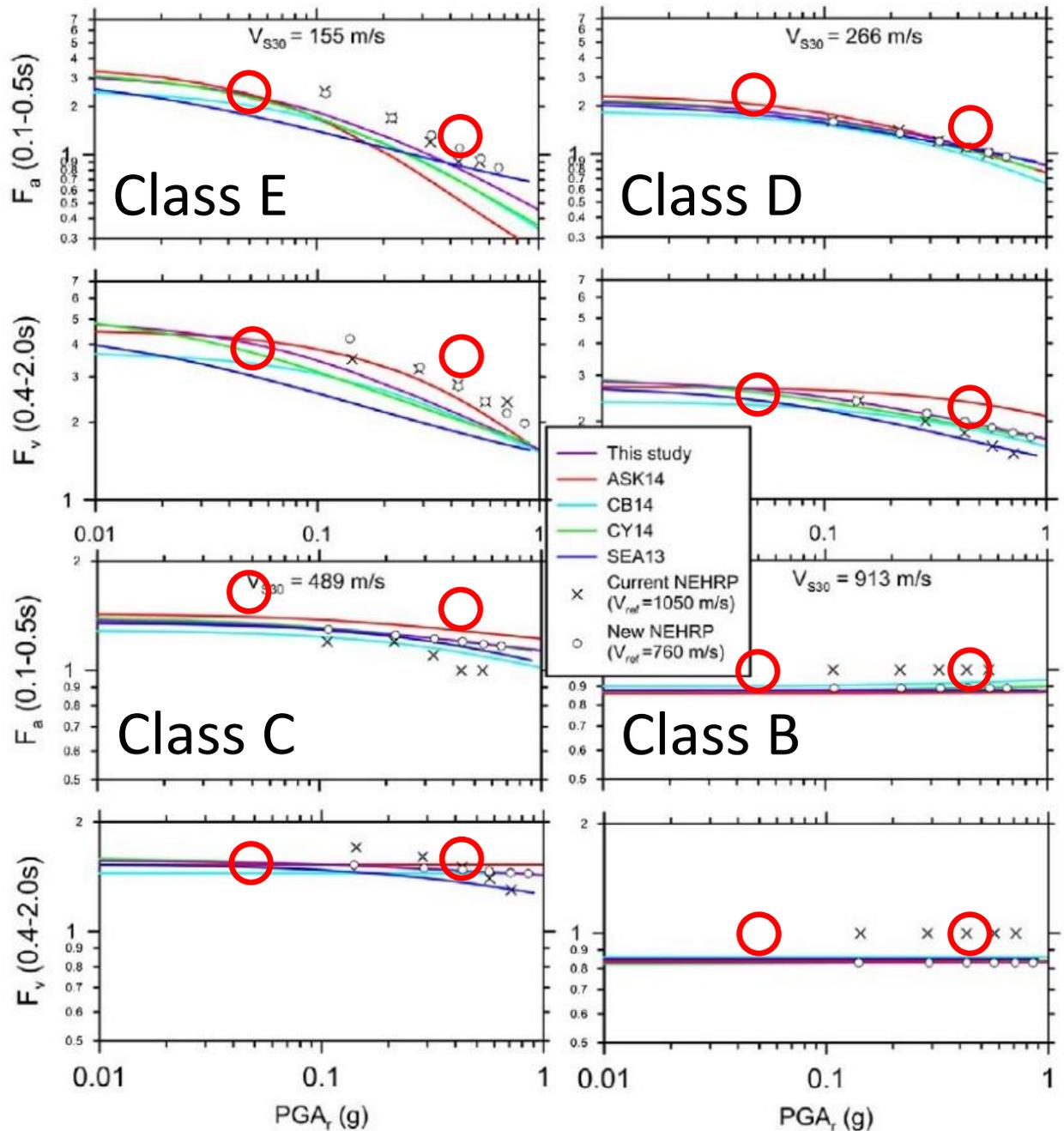
To examine the amplitude dependence of the site factors more quantitatively, we are evaluating the amplification factors using records observed at nearby station pairs (Hori and Midorikawa, 2016).
