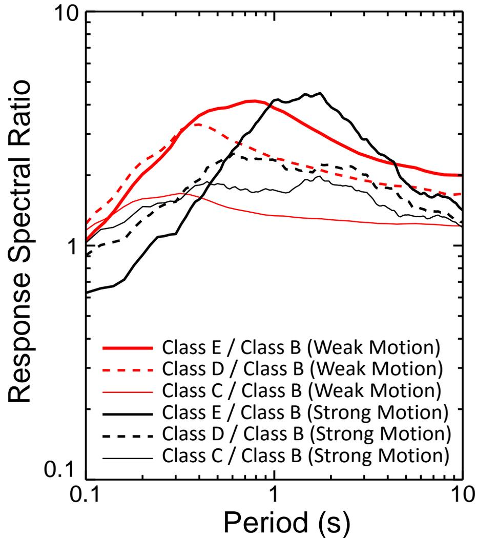
The amplifications evaluated for weak motion are shown by red lines. In general, the amplification from strong motion is smaller at short periods and larger at longer periods than that from weak motion. The difference in both amplifications is smaller at site class C (stiff site) and larger at site class E (soft site).
