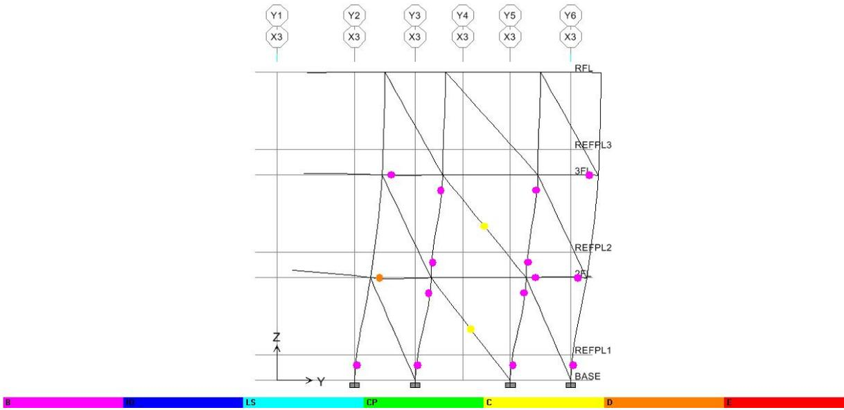
圖 C.78 Y 向之 X3 Frame(Deformed Shape-by PushX Static Nonlinear)
