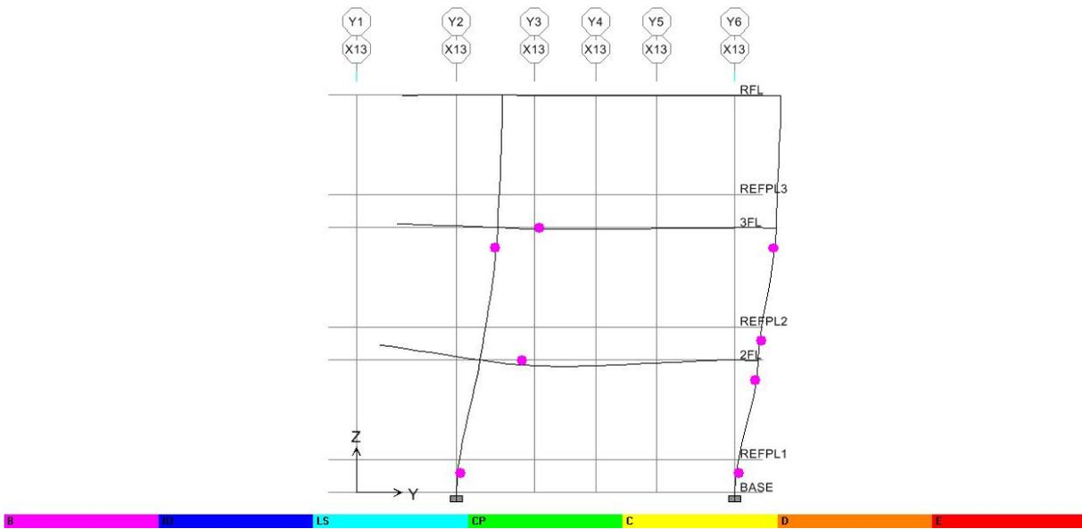
圖 C.88 Y 向之 X13 Frame(Deformed Shape-by PushX Static Nonlinear)
