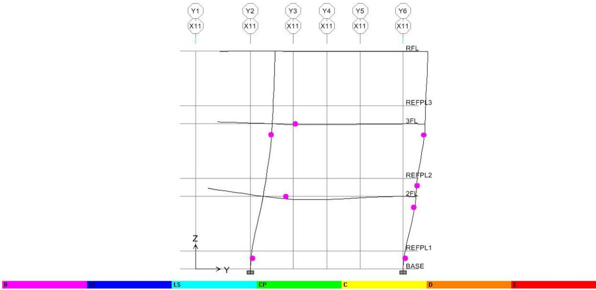
圖 C.86 Y 向之 X11 Frame(Deformed Shape-by PushX Static Nonlinear)
