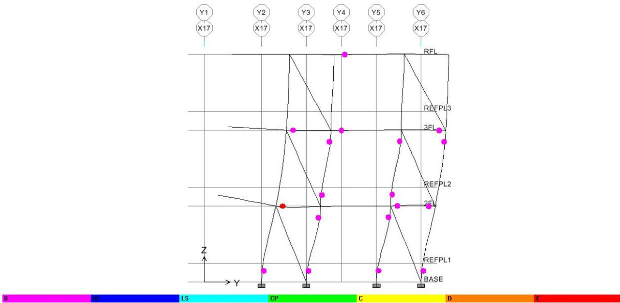
圖 C.92 Y 向之 X17 Frame(Deformed Shape-by PushX Static Nonlinear)
