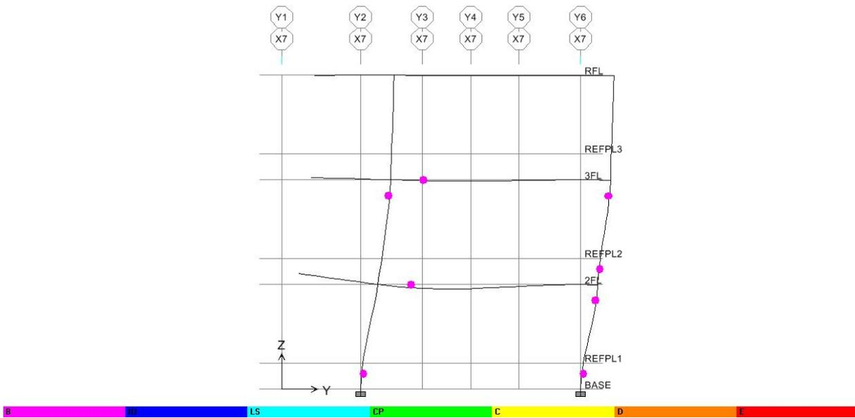
圖 C.82 Y 向之 X7 Frame(Deformed Shape-by PushX Static Nonlinear)
