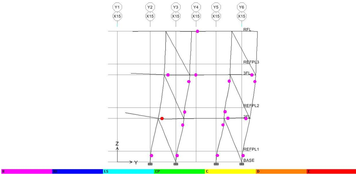
圖 C.90 Y 向之 X15 Frame(Deformed Shape-by PushX Static Nonlinear)
