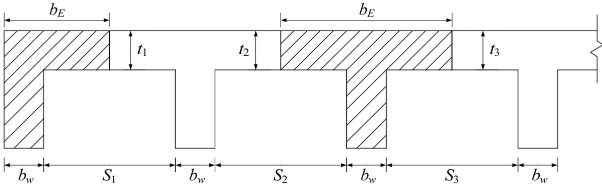
$$\text{雙翼 T 型梁： } b_E = \min(L/4, b_w + \min(8t_2, \frac{S_2}{2}) + \min(8t_3, \frac{S_3}{2}))$$
