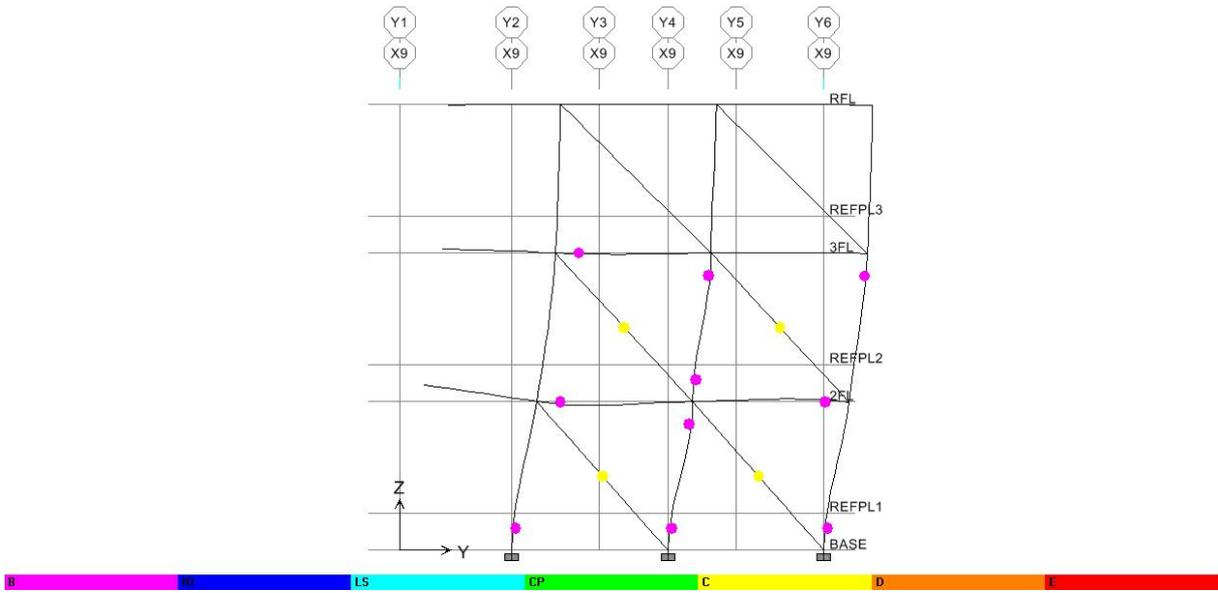
圖 C.84 Y 向之 X9 Frame(Deformed Shape-by PushX Static Nonlinear)
