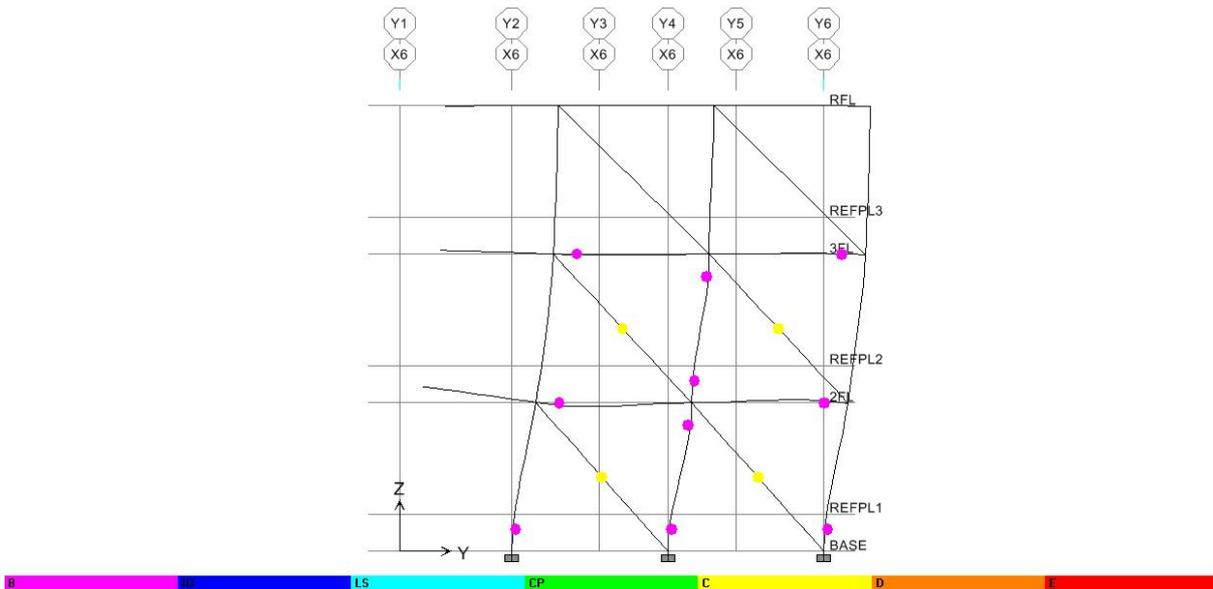
圖 C.81 Y 向之 X6 Frame(Deformed Shape-by PushX Static Nonlinear)
