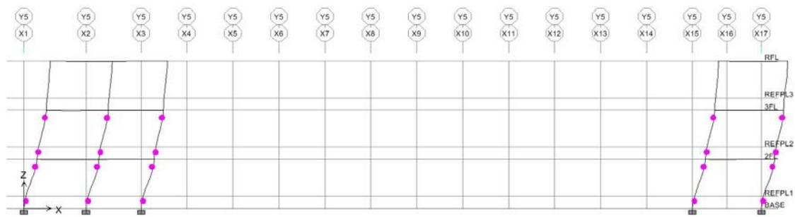
圖 C.67 X 向之 Y5 Frame(Deformed Shape-by PushX Static Nonlinear)
