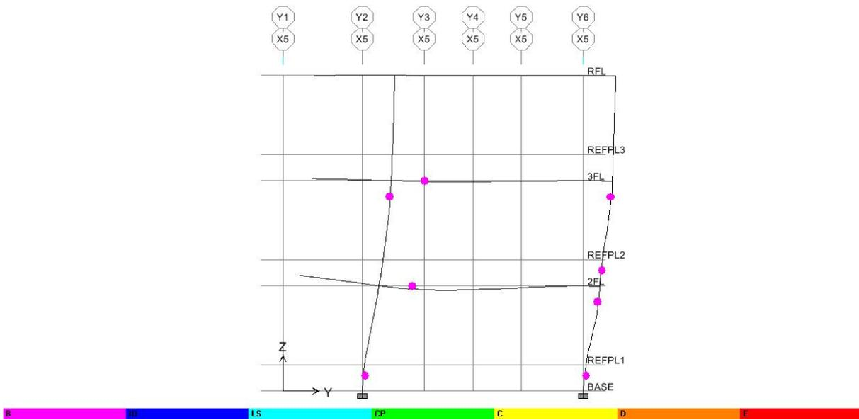
圖 C.80 Y 向之 X5 Frame(Deformed Shape-by PushX Static Nonlinear)
