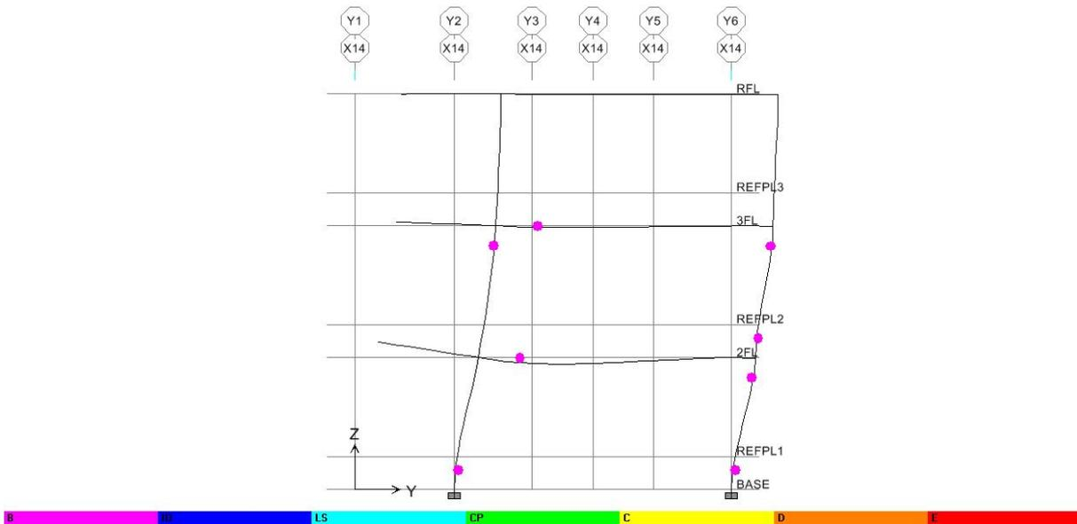
圖 C.89 Y 向之 X14 Frame(Deformed Shape-by PushX Static Nonlinear)
