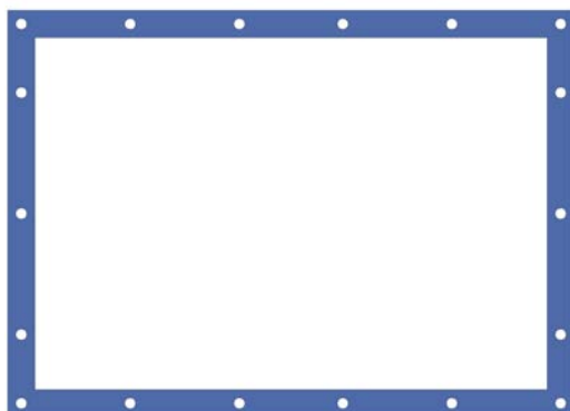
Figure 6. The clamping strip for fixing the base board.
