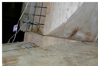
試體 CC2 於 drift15%, cycle1, pull
