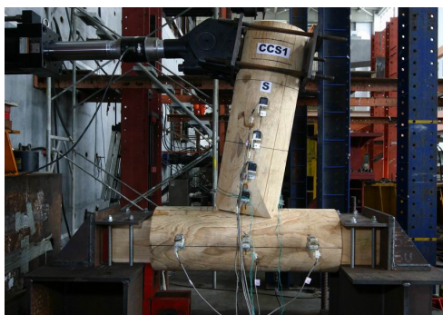
試體 CCS1 於 drift15%, cycle1, push
