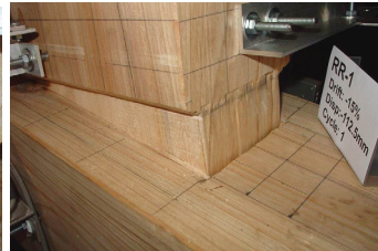
試體 RR1 於 drift15%, cycle1, pull
