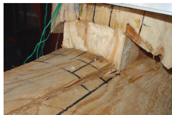
試體 CCS1 於 drift15%, cycle2, pull
